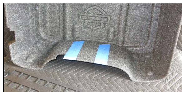
Masking tape with hole locations marked.
