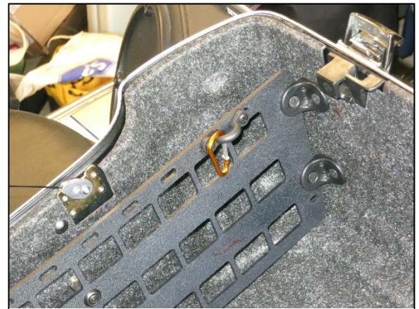
The tool loop installed. Carabiner not provided. Image shows tool loop on TP-3.09s. All TACTICAL PANELS similar.
